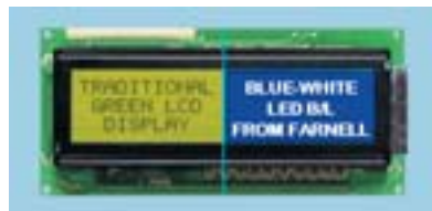
Photograph to show difference between standard LCD and the Blue-White LCD
